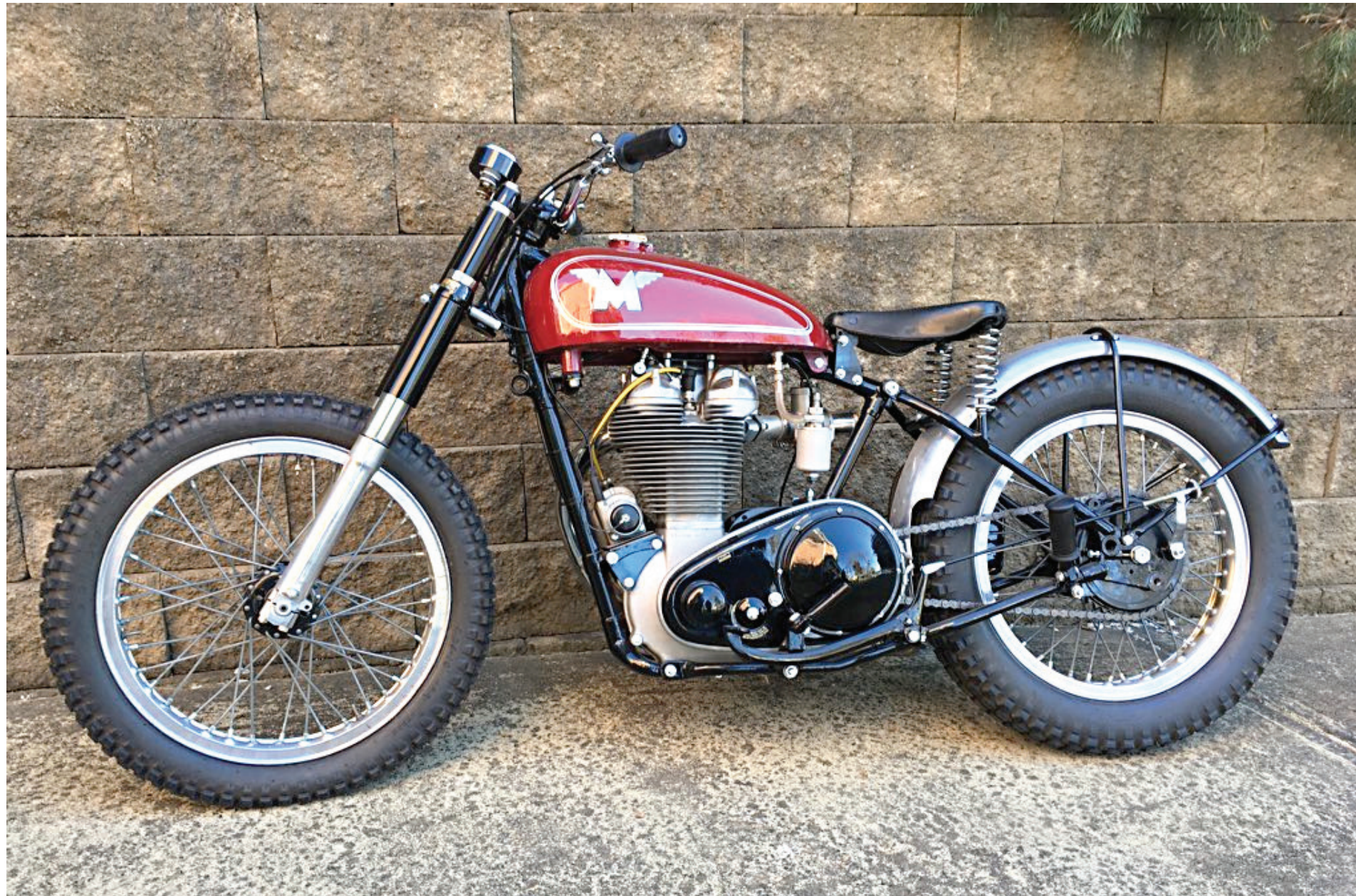
Lean and mean - off-side view shows special folding foot pegs and rear brake and pedal which were removed for Class C racing.
