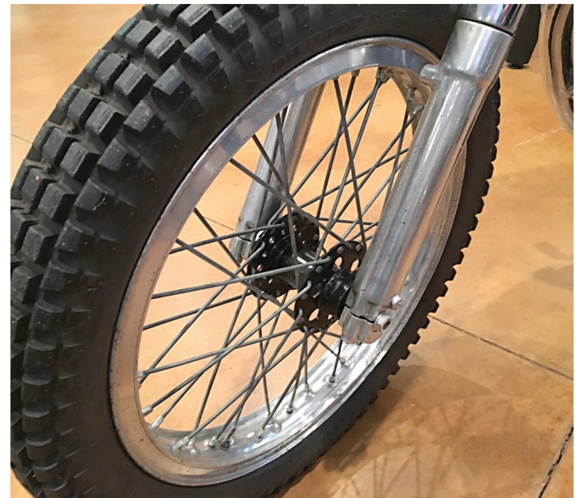
Dunlop alloy rims came standard. Front spool hub is early model rear hub ...
