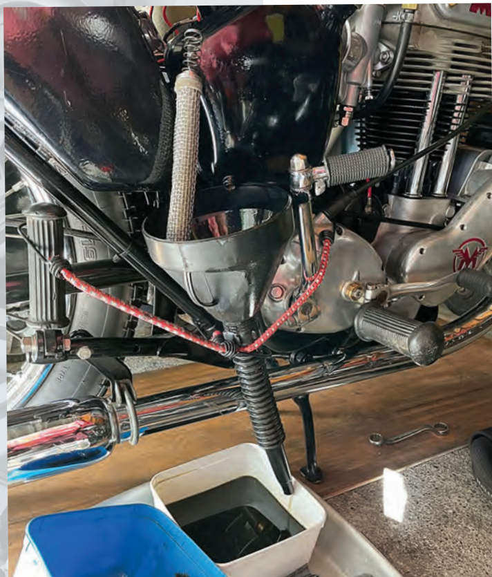
Gearbox oil topped up to the level hole
