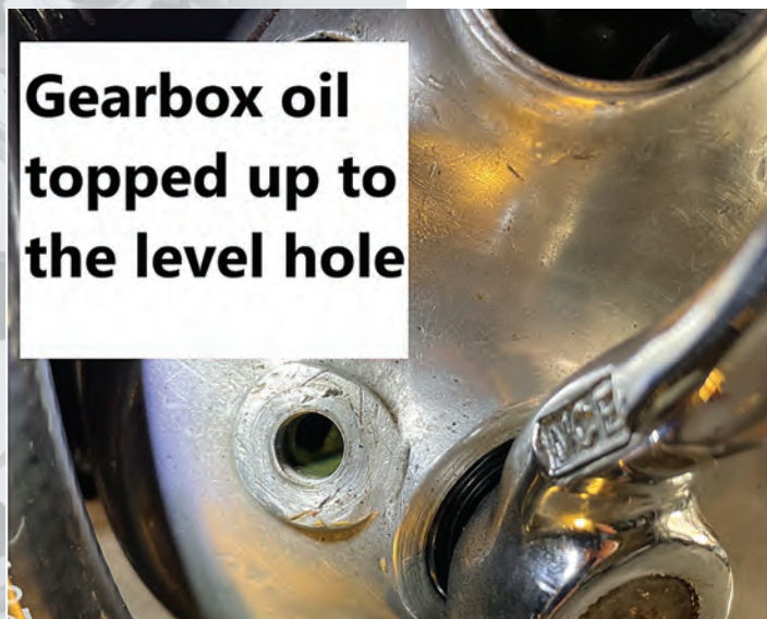
Fresh oil added up to the level of the inspection hole
