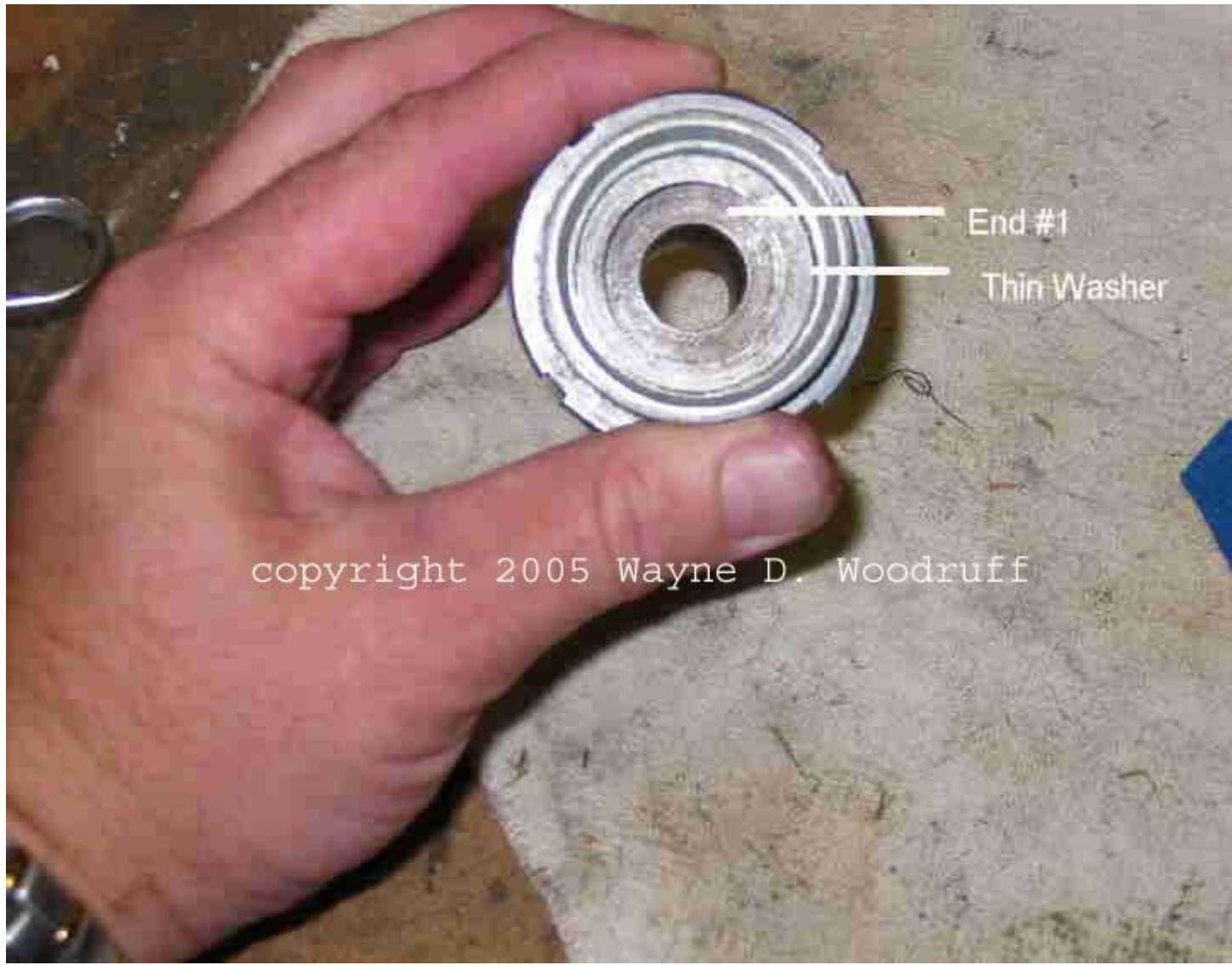
Fig 4: The thin washer (4th from left in 1st photo) now in place
