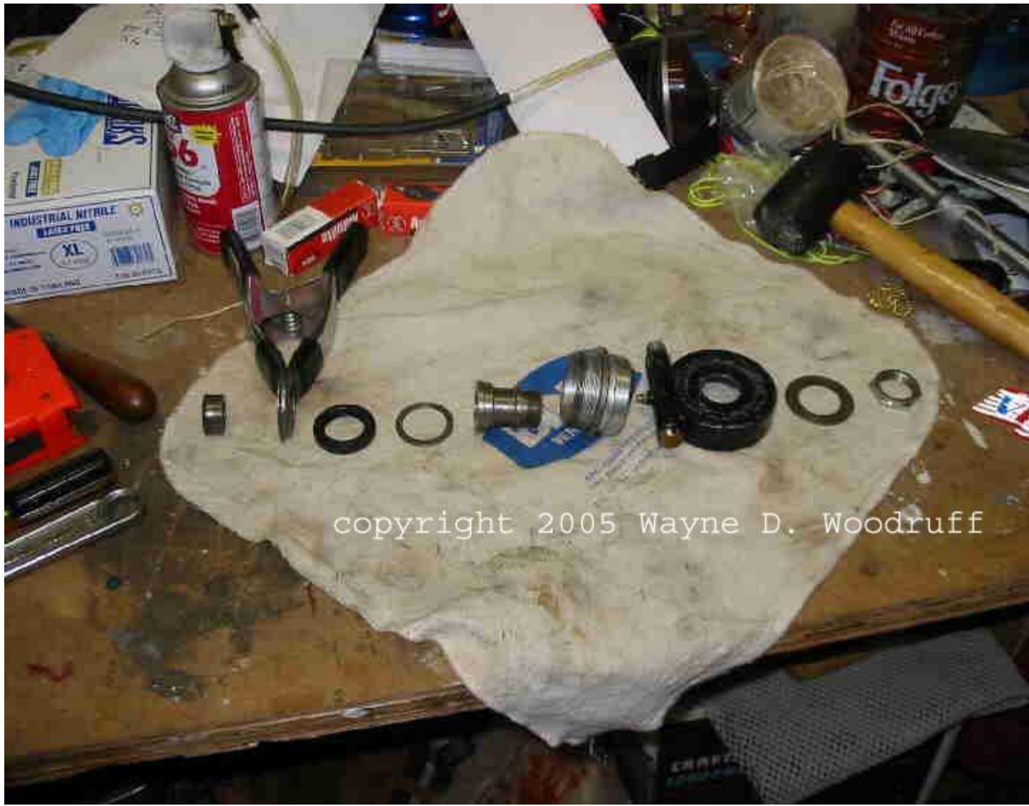
Fig 1: All parts laid out in the proper sequence and proper orientation. Pay particular attention to the orientation of the seal cup (2nd part from the left). The "wide" side faces AWAY from the seal!
