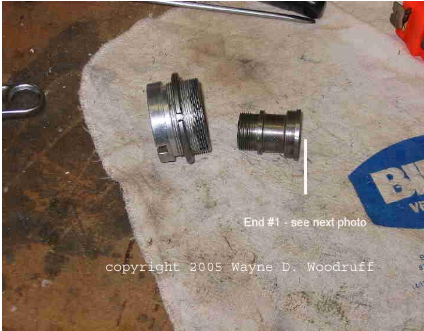
Fig 2: The threaded axle the speedo drive attaches to as about to be inserted in the retaining ring
