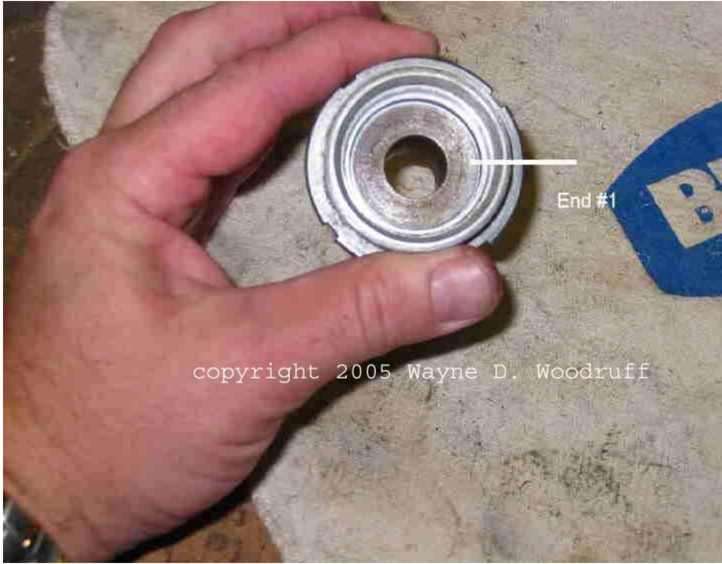
Fig 3: End view of Fig 2. The threaded axle now rests in the seat
